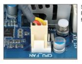
Step 5: Finally, attach the power connector of the CPU cooler to the CPU fan header (CPU\_FAN) on the motherboard.
