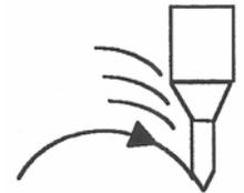
G2 moves in a clockwise circular motion, and G3 moves in a counterclockwise circular motion. This clockwise and counterclockwise motion is relative to your point of view, however. See the diagram below. The X, Y or Z position specified in the G2 or G3 command is the end position of the arc, and may be an absolute position (G90) or an incremental position (G91). G2 and G3 are modal and remain in effect until another positioning mode (G0, G1, etc.) is commanded.
